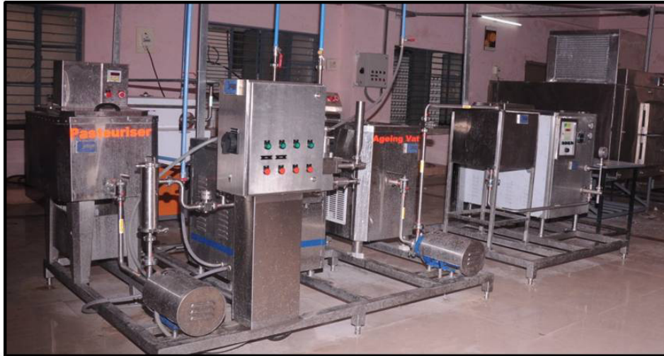
Continuous Ice-cream making unit(400 cups per Hour) Cost : Rs. 24 lakhs
